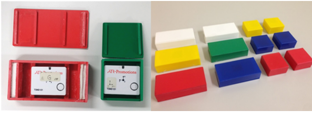
Figure 2: Toy blocks with the embedded IMU-sensors
